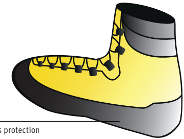
Crampon midsole made of TPU with differentiated diameter in the ball
